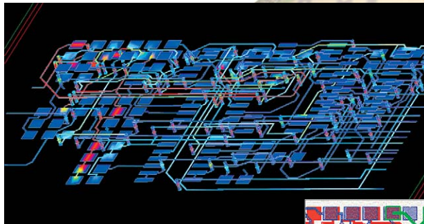
ADS Layout information is combined with the Momentum substrate definition to produce a 3D spatial representation of circuit geometries.
